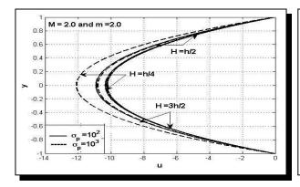
**Figure 12.** Secondary velocity w for M = 2.0, m = 1.0 and different values of H
