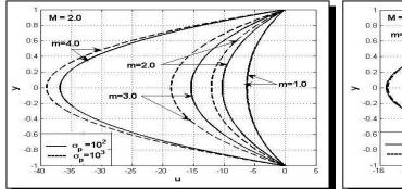
**Figure 8.** Secondary velocity w for M = 2.0 and different values of m
