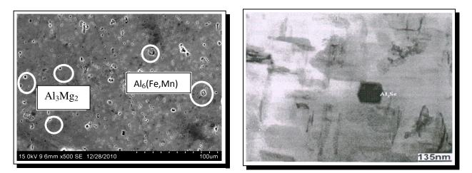
Figure 3. AA5083-H321 SEM Microstructure [11] Figure 4. Cast Al-Mg-Sc TEM Microstructure [12]
