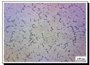
Figure 2. Cast Al-Mg-Sc Base Metal
