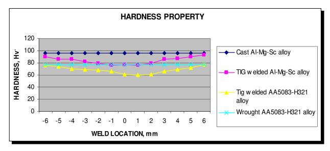
Figure 11. Variation of Hardness of TIG welded samples and their Base metals
