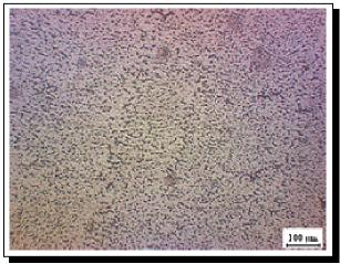
Figure 8. Weld microstructure of TIG weld
