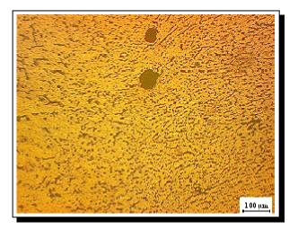
**Figure 7.** Porosity at the HAZ of the TIG welds
