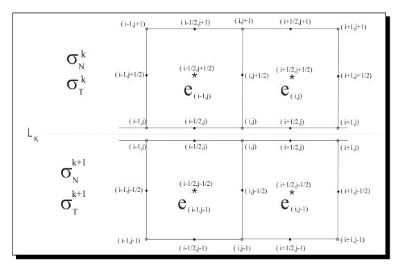
Figure 2. The interlayer finite elements
