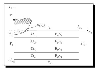
Figure 1. Geometry of the spherical indentation
