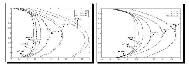
**Figure 2.** Axial velocity,  $u(\xi)$  for  $\bar{\alpha} = 0.1$  and  $\sigma_1 = 10^1$  and different values of *M*
