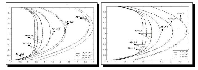
**Figure 6.** Axial velocity,  $u(\xi)$  for  $\bar{\alpha} = 0.1$  and  $\sigma_2 = 10^1$  and different values of *M*
