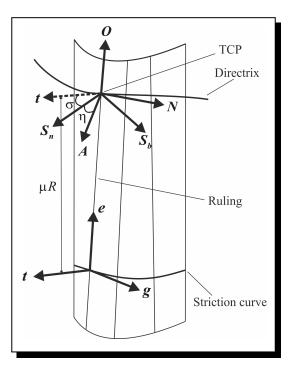
**Figure 3.** Relations between three reference frames as a robot end-effector moves on a specified trajectory.
