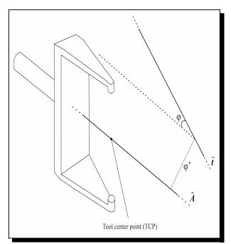
**Figure 5.** The dual angle between the dual unit vectors  $\tilde{A}$  and  $\tilde{t}$ .
