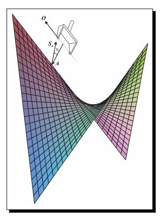
Figure 6. A robot end-effector which moves on the surface of a hyperbolic paraboloid.
