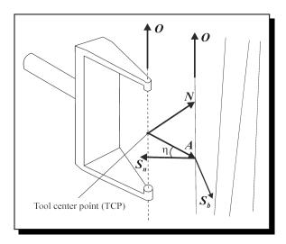
Figure 2. The spin angle which is the angle between approach vector and the surface normal vector.
