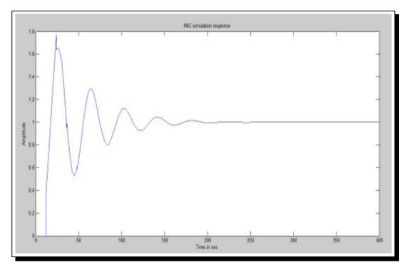
Figure 11. IMC Closed Loop Response
