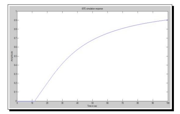
Figure 17. Integral of Square Time Error Closed Loop Response
