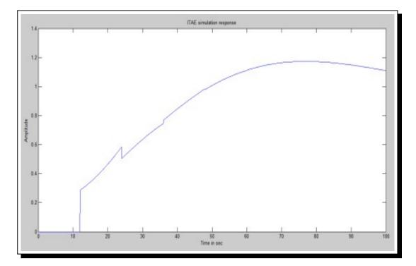
Figure 15. Integral of Time Absolute Error Closed Loop Response
