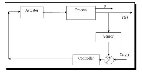
Figure 3. Basic closed loop systems
