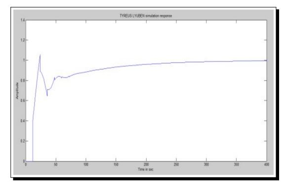
Figure 12. TyreusLyuben Closed Loop Response
