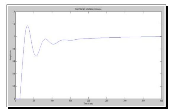
Figure 13. Gain Phase Margin Closed Loop Response
