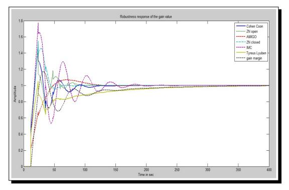
Figure 4. Robustness Response of the Gain Value
