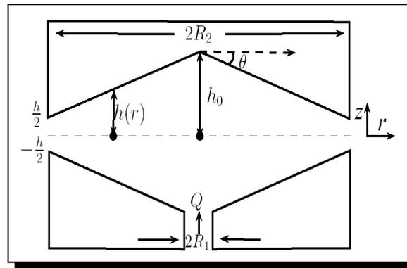
Figure 1. Geometry of an externally pressurized convergent thrust bearing
