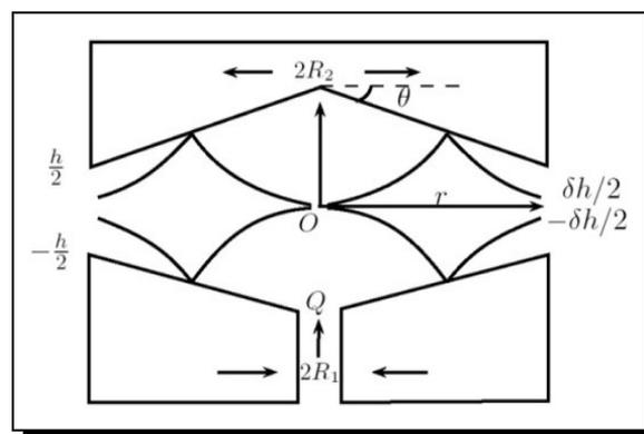
Figure 2. Shape of the core in an externally pressurized convergent thrust bearing
