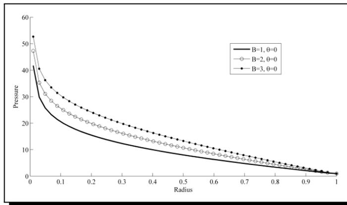
**Figure 3.** Pressure distribution for different angles of convergence
