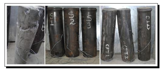
Figure 2. Specimens after buckling
