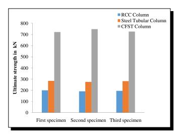
Figure 7. Comparison between the ultimate strength of the HAST, RCC and CFST columns
