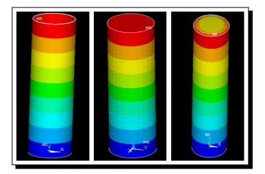
Figure 5. Nodal solutions of the HST, RCC and CFST columns
