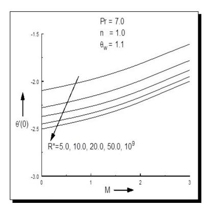
**Figure 10.** Dimensionless rate of heat transfer for different  $R^*$
