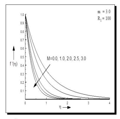
Figure 2. Velocity profiles for different *M*
