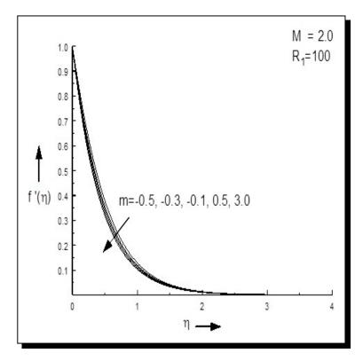
Figure 1. Velocity profiles for different *m*
