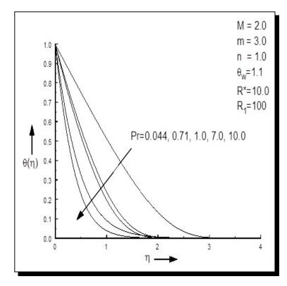
Figure 4. Temperature profiles for different Pr
