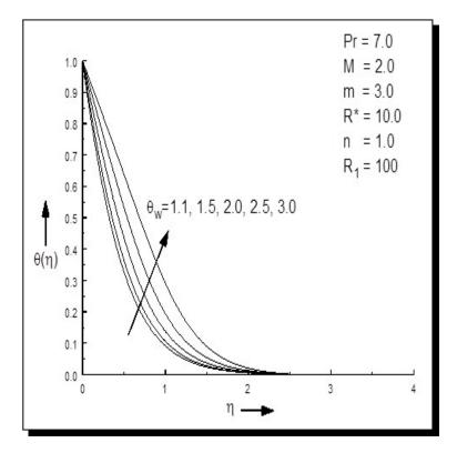
**Figure 7.** Temperature profiles for different  $\theta_w$
