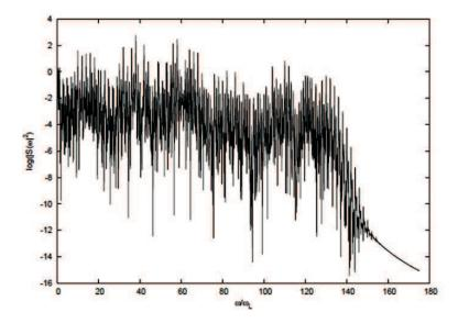
Figure 2. The HHG Spectrum of the QD when shined by a laser pulse of intensity 224.65 TW/cm<sup>2</sup>.
