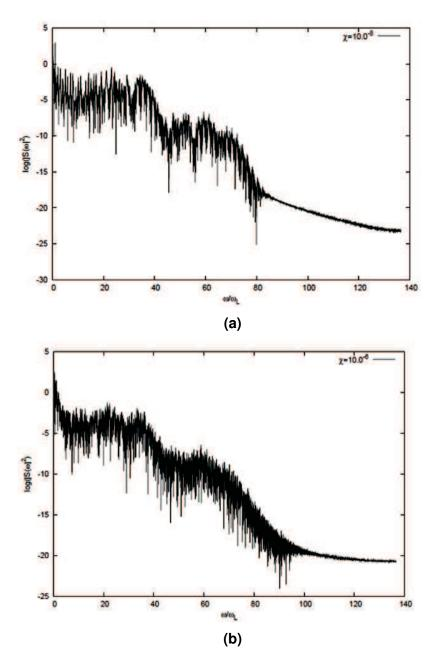
**Figure 3.** The HHG Spectrum of the QD when shined by a laser pulse of intensity  $87.77 \text{ TW/cm}^2$  with chirping rate (a)  $1.2418 \times 10^{-21} \text{s}^{-2}$  (b)  $1.2418 \times 10^{-19} \text{s}^{-2}$ .
