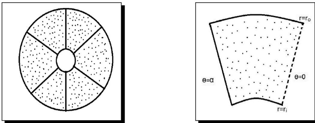
(a) Cross-sectional view of concentric pipes (b) Computational domain
