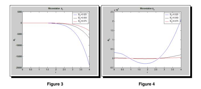
It is observed from Figure 3 that the microrotation component  $\varphi_r$  is constant for various values of  $B_3$  when r < 1.5 and decreases gradually for r > 1.5. Figure 4 shows that microrotation component  $\varphi_z$  decreases when r < 1.7 and increases from there.
