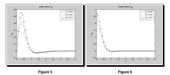
It is observed from Figure 5 that couple stress component  $m_{zr}$  rapidly increases r < 0.3 and rapidly decreases between 0.3 < r < 1 and then it is constant almost when distance is greater than 1. Similarly other couple stress component  $m_{zz}$  decreases rapidly when r < 1 and almost constant from there onwards in Figure 6.
