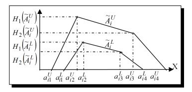
Figure 1. The upper trapezoidal MF $\tilde{\tilde{A}}_{i}^{U}$  and the lower MF $\tilde{\tilde{A}}_{i}^{L}$  of the IT2 FS $\tilde{A}_{i}$
