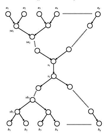
**Figure 3.** Propagation of vertical constraints from p sink nets of group A to q source nets of group B through bounded degree separator nets.
