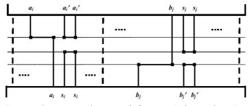
**Figure 2.** The constructed instance I' of two-terminal nets, where (i)  $a_i$  and  $a'_i$  are to be assigned to the same track, (ii)  $b_j$  and  $b'_j$  are to be assigned to the same track, and (iii)  $s_i$  and  $s_j$  are to be assigned to the same track.
