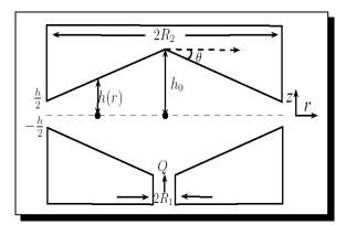
Figure 1. Geometry of an externally pressurized convergent thrust bearing
