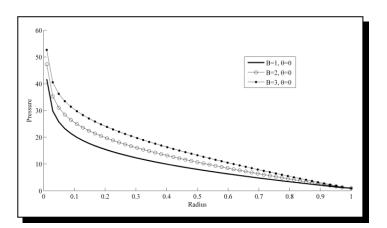
Figure 3. Pressure distribution for different angales of convergence
