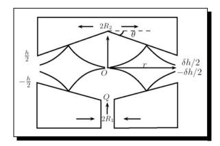
Figure 2. Shape of the core in an externally pressurized converging thrust bearing
